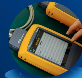
Fluke DSX Certification Testing
